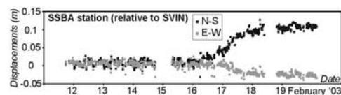
**Figure 2.** Ten-minute average values of 1 Hz displacement time series of the SSBA station from the start of operations on 11 February until a lava flow destroyed it on 20 February. Data gaps are due to radio communication outages.
