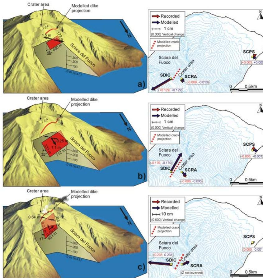
**Figure 3.** Three-dimensional model sketches and observed-model displacement vectors of the Sciaradat network and CGPS station SCPS on the volcano's base during the 5 April explosion, for the a) first phase of the explosion; b) second phase; c) final phase.
