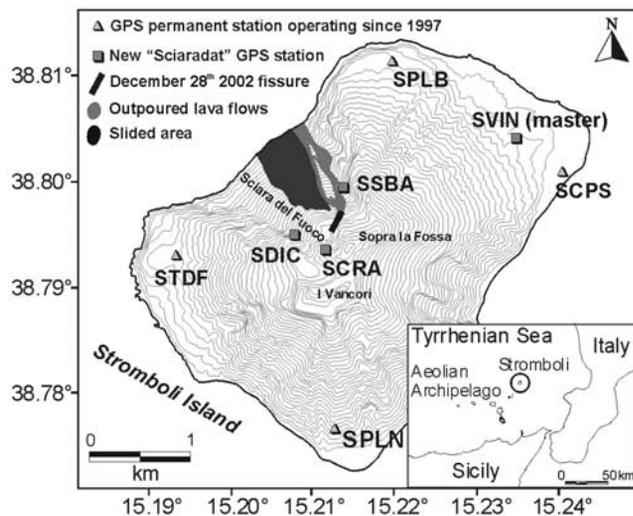
**Figure 1.** Continuous GPS monitoring stations on Stromboli Island.
