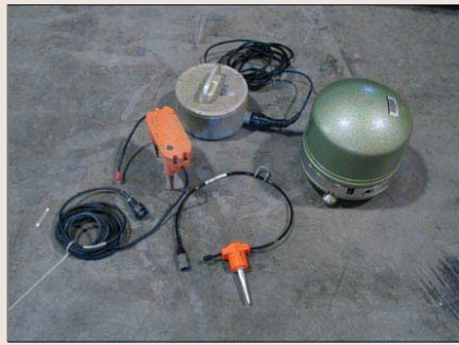
Figure 3. Members of the PASSCAL family of sensors. Clockwise from the top: Silver sensor = three-component L-22 with a natural period of 2 Hz; green sensor = Strekheisen STS-2 broadband sensor with a frequency response shown by the yellow line in Figure 2; orange single component 40-Hz geophone; and three-component 4.5-Hz geophone similar to those used in the exploration industry. Responses are shown in Figure 2.
