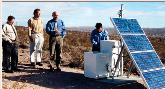
Figure 8. A completed PASSCAL-style installation. This site is actually a prototype USArray installation near the PASSCAL Instrument Center in Socorro, New Mexico.
