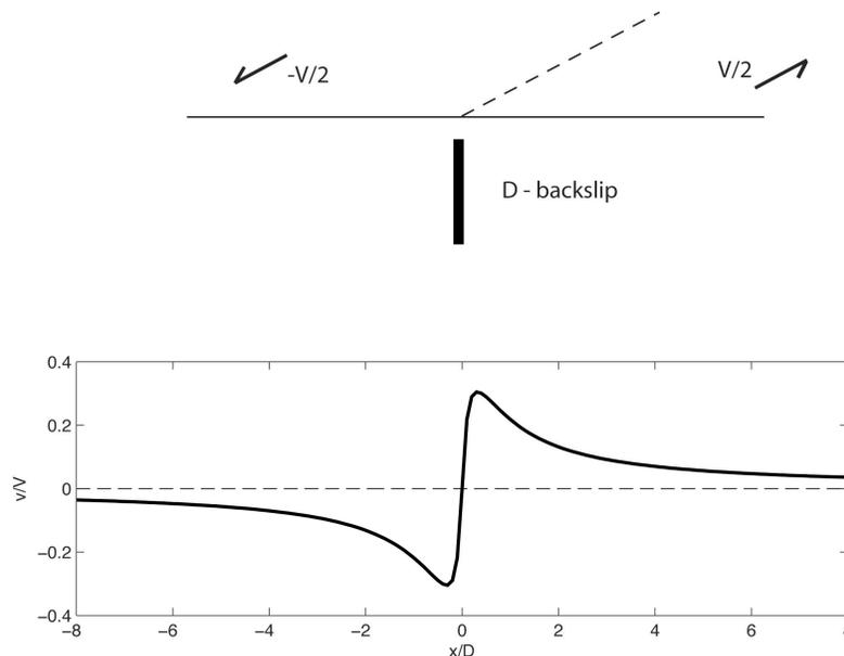
Schematic of surface velocity due to uniform backslip rate over a depth  $D$ .
