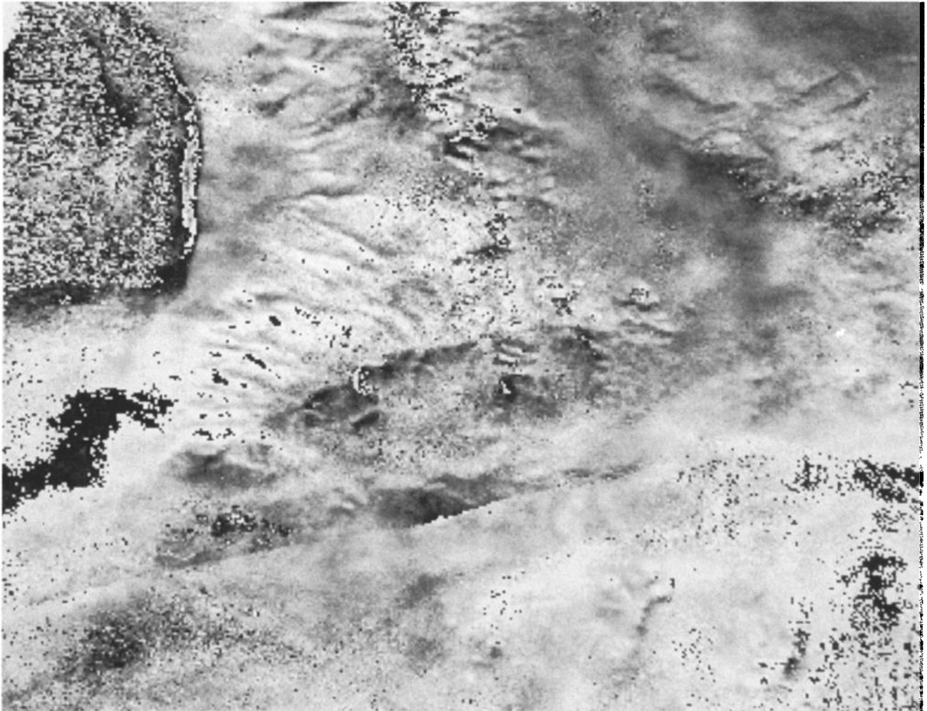
Figure 10. An interferogram showing surface rupture on the Garlock fault in California, as well as some artificial residuals. The surface rupture appears in all the coseismic interferograms of Landers. It represents 7 \pm 4 mm of range change, projected as 19 \pm 10 mm on the ground, assuming pure horizontal displacement. Data from Massonnet et al. [1994a] as described in the caption for Plate 20a. One complete cycle of shading (from solid black to solid white) corresponds to 28 mm of range change.
