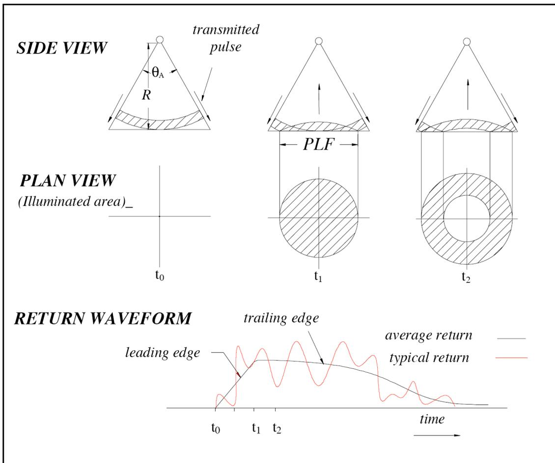
$0 < t < t_0$  pulse propagates as part of expanding spherical shell. Area of sphere that can be received on ground defined by antenna beamwidth ( $\theta_A$ )
