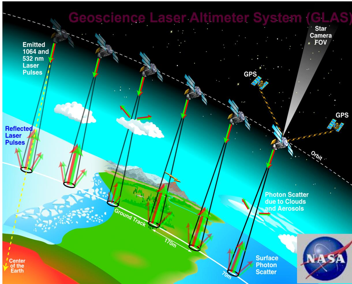
**Schematic of single profile science data measurements, compiled through time to build elevation data sets**
