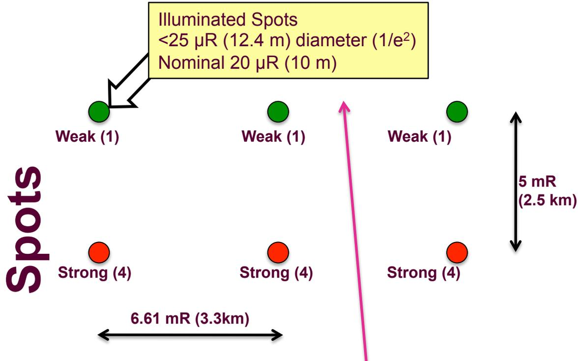
Weak & strong spots maximize the penetration of a given total laser energy
