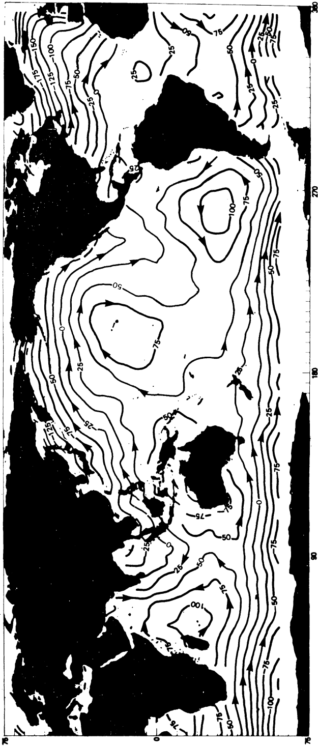
Fig. 14. Dynamic topography determined from altimetry. Contours in centimeters represent the difference between a long-term mean sea surface and a global geoid model. The surface consists of 1.5 years of GEOS-3 data plus all existing SEASAT altimetry. The geoid model, called PGS-54 is based on a combination of satellite observational data, surface gravity, and also altimeter data. Both surfaces were smoothed before performing the difference to reveal only the large-scale (> 10,000 km) circulation features. Although certain aspects of the map are probably unrealistic, based on comparison with dynamic height maps from hydrography, gyres with the correct sense are found in the major ocean basins. A strong Antarctic Circumpolar Current is also apparent. [From Cheney and Marsh (1982).]
