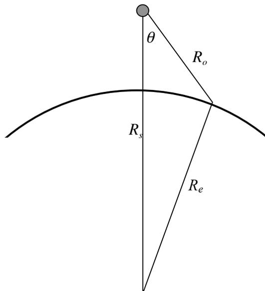
This diagram has the satellite at the gray dot with the velocity vector pointing into the page. The cosine of the look angle is
