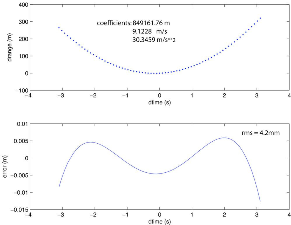
1) The first thing learned is that the parabolic approximation to a hyperbola used in the SAR processor has a maximum error of about 1 cm at a time offset of 3 seconds. This corresponds to a small fraction of the 23-cm wavelength. Note that the actual aperture length for ALOS is only +/- 1.5 seconds so this approximation is justified.
