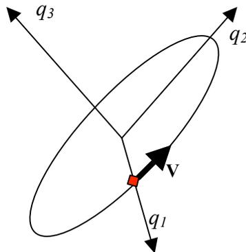
In this primed co-ordinate system, the  $q_1$ -axis is parallel to  $\vec{R}_s$ , the  $q_2$  axis is parallel to  $\vec{V}$ , and the  $q_3$  axis is perpendicular to both and is given by their cross product
