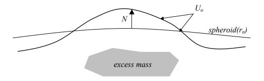
Because of the excess mass, the potential on the spheroid is higher than the reference level  $U = U_o + \Phi$ . Thus, the ocean surface must move further from the center of the earth to remain at the reference level  $U_o$ . To determine how far it moves, expand the potential in a Taylor series about the radius of the spheroid at  $r_o$ .
