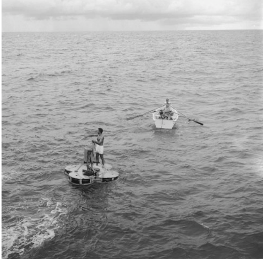
Figure 6. Willard Bascom on instrument raft, John Isaacs and Monk Hendrix in the rowboat. Four truck inner tubes are used for floatation of the plywood raft, which was anchored to the 4500 ft deep seamount by San Diego trolley car wheels.
