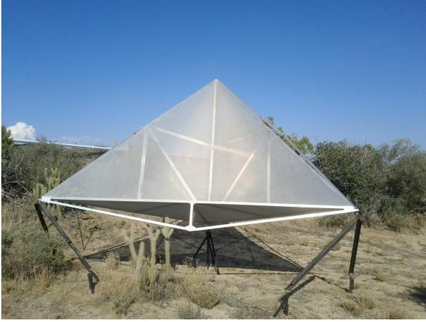
**Figure 4** One of the 2.4 m radar corner reflectors at Pinon Flat Obs. installed in 1998 (photograph taken September 12, 2012). This arid region, at an elevation of 1200 m, is relatively flat with a surface of decomposed granite sparsely covered by bush and grass. Three radar corner reflectors are oriented to reflect energy from ascending (A1) and descending (D1 and D2) ALOS passes.
