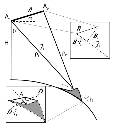
**Figure 1** Imaging geometry of side-looking radar for InSAR applications. The *box* in the *top right* illustrates the contribution of the orbit separation baseline to measured range differences. The *box* in the *bottom left* illustrates the range change caused by the surface displacement component in the range direction. See text for discussion and explanation.
