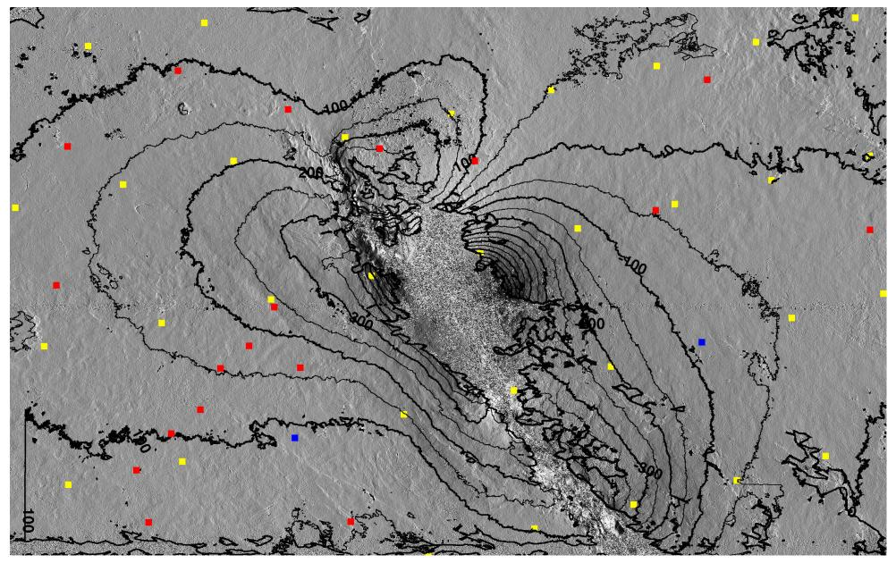
Contours of line-of-sight displacement (mm) superimposed on east component of phase gradient for Hector Mine 7.1 M Earthquake. red - gps locations blue - 1/2 degree ticks (mapped into radar co-ordinates)
