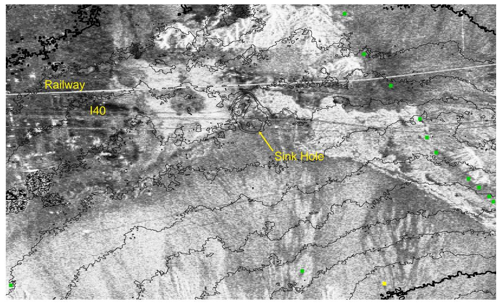
Contours of line-of-sight displacement (10 mm interval) superimposed on radar amplitude. Interstate 40 passes over a 30 mm deep, 1000 m diamterer sink hole . This area is just east of Barstow CA. yellow - 1/8 degree ticks (mapped into radar co-ordinates)
