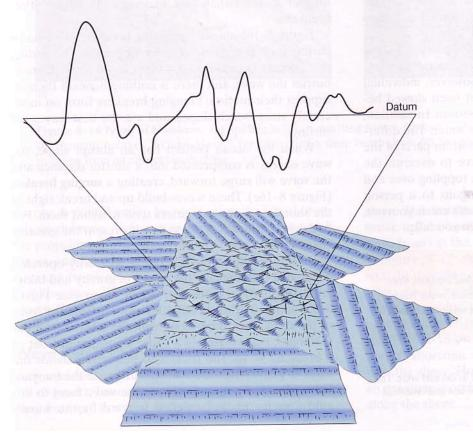
Figure 8-14 Mixed interference pattern. The observed wave pattern in the ocean (above) is often the result of mixed interference of many different overlapping wave sets (below).
