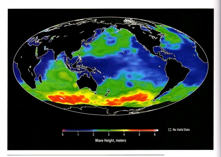
Figure 8-10 TOPEX/Poseidon wave height, October 3-12, 1992. The TOPEX/Poseidon satellite receives a return of stronger signals from calm seas and weaker signals from seas with large waves. Based on these data, a map of wave height can be produced. The largest average wave heights (red areas) are in the prevailing westerly wind belt in the Southern Hemisphere. (Scale in meters.)
