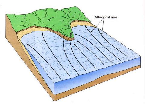
The long black arrows in Figure 8-18 are called orthogonal (ortho = straight, gonia = angle) lines. Orthogonal lines are drawn perpendicular to the wave fronts (so they indicate the direction that waves travel) and are spaced so that the energy between lines is equal at all times. They help determine how energy is distributed along the shoreline by breaking waves.
