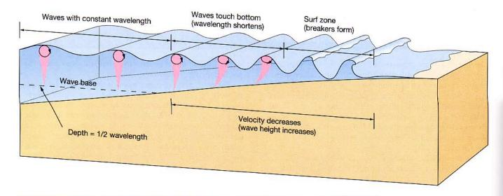
Figure 8–15 Physical changes of a wave in the surf zone. As waves approach the shore and encounter water depths of less than one-half wavelength, the waves "feel bottom." The wave speed decreases and waves stack up against the shore, causing the wavelength to decrease. This results in an increase in wave height to the point where the wave steepness is increased beyond the 1:7 ratio, causing the wave to pitch forward and break in the surf zone.
