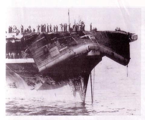
Figure 8-12 Wave damage on the aircraft carrier Bennington. The Bennington returns from heavy seas encountered in a typhoon off Okinawa in 1945 with part of its reinforced steel flight deck bent down over the bow. Damage to the flight deck, which is 16.5 meters (54 feet) above still water level, was caused by large waves.
