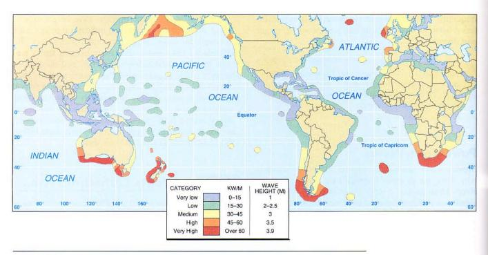
Figure 8-24 Global coastal wave energy resources. Distribution of coastal wave energy shows that more wave energy is available along western shores of continents, especially in the Southern Hemisphere. KW/M is kilowatts per meter (for example, every meter of "red" shoreline is a potential site for generating over 60 kilowatts of electricity); average wave height is in meters.
