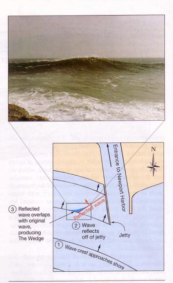
Figure 8-19 Wave reflection at The Wedge, Newport Harbor, California. As waves approach the shore (1), some of the wave energy is reflected off the long jetty at the entrance to the harbor (2). The reflected wave overlaps and constructively interferes with the original wave (3), resulting in a wedge-shaped wave (dark blue triangle) that may reach heights exceeding 8 meters (26 feet). Photo of The Wedge (inset) shows three dots in front of the wave that are the heads of body surfers.
