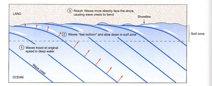
Figure 8-17 Refraction along a straight shoreline. Waves approaching the shore at an angle first "feel bottom" close to shore. This causes the segment of the wave in shallow water to slow, causing the crest of the wave to refract or bend so that the waves arrive at the shore nearly parallel to the shoreline. Red arrows represent direction and speed of the wave.
